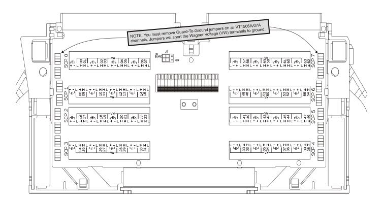
Figure 5. VT1506A/07A C-Size Terminal Module Connections
