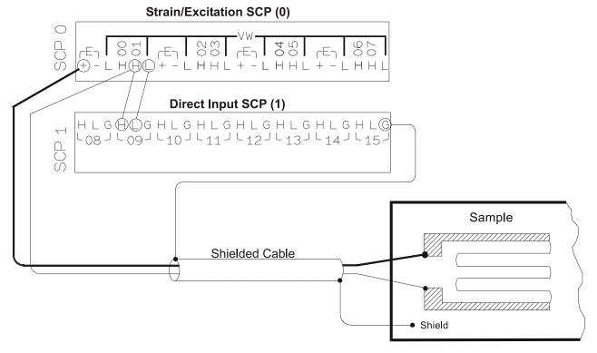
Figure 10. Typical 1/4 Bridge Connections
