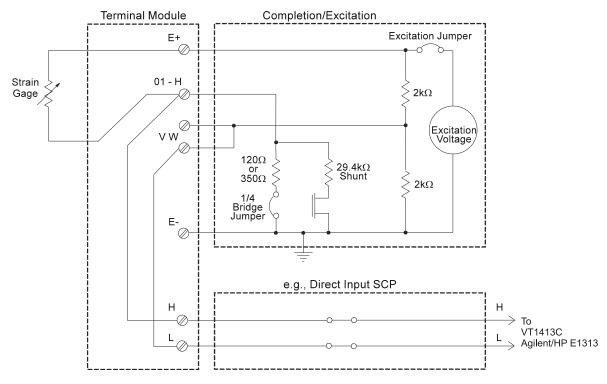
Figure 1. Typical 1/4 Bridge Strain Gage Measurement
