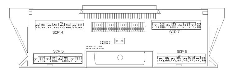
Figure 7. VT1506A/07A B-Size Terminal Module Connections (Ch. 32 - 63)
