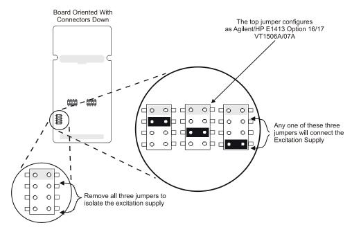
Figure 15. Isolating the Internal Excitation Supply
