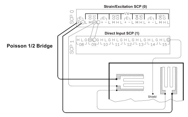
Figure 11. Typical 1/2 Bridge Connections
