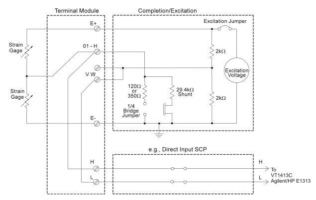
Figure 2. Typical 1/2 Bridge Strain Gage Measurement
