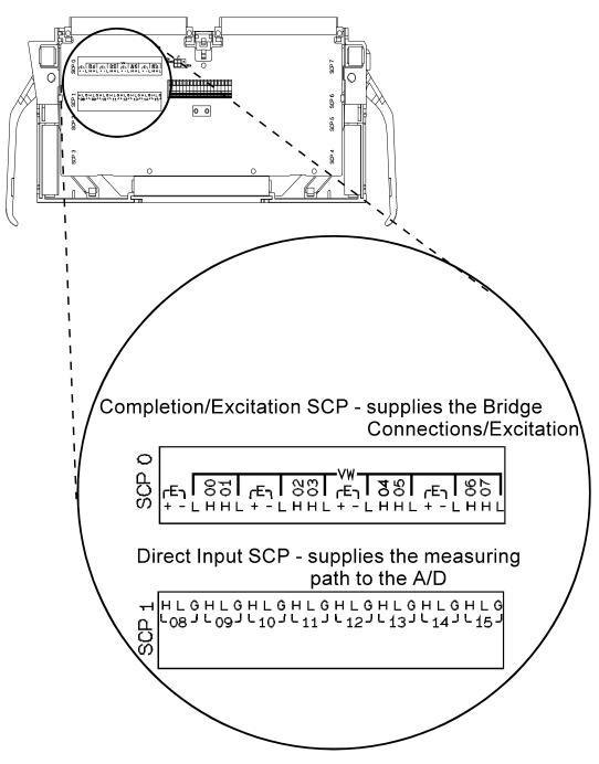
Figure 9. Typical Locations of Terminal Module Connections
