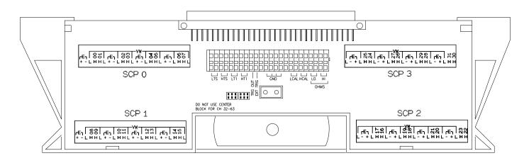
Figure 6 . VT1506A/07A B-Size Terminal Module Connections (Ch. 00 - 31)
