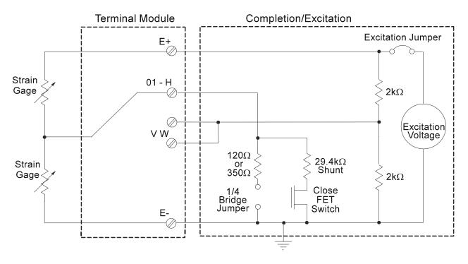
where 1 or ON adds the shunt resistor and 0 or OFF (default value) removes the resistor.
