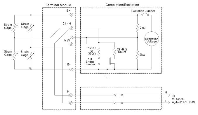
Figure 3. Typical Full Bridge Strain Gage Measurement
