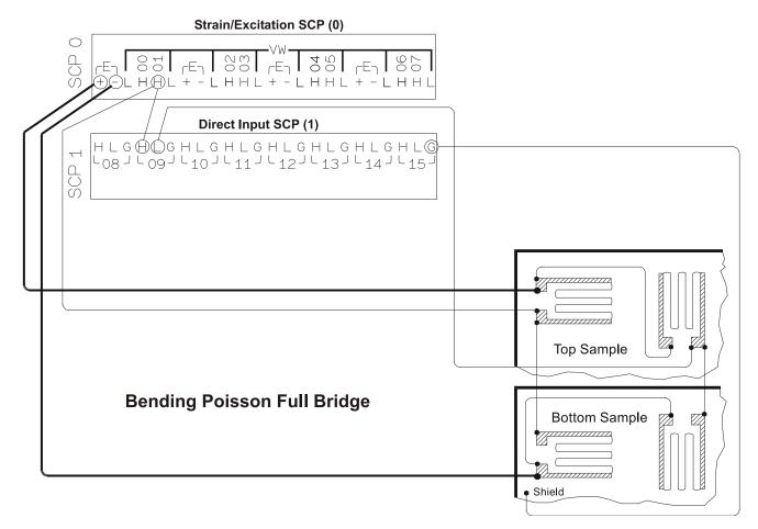
Figure 13. Full Bridge Connections (Cont.)
